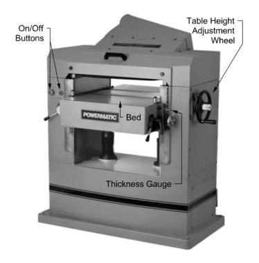
The planer is used to smooth lumber to an even thickness. After flattening one side of a board on the jointer, the board is run through the planer with the flat side down on the table, which supports the board and acts as a reference surface. The cutterhead, located above the workpiece, then smoothes the opposite face and makes it parallel to the jointed face. The width of the cutterhead, which defines the size of a planer, indicates the widest board that can be surfaced.
