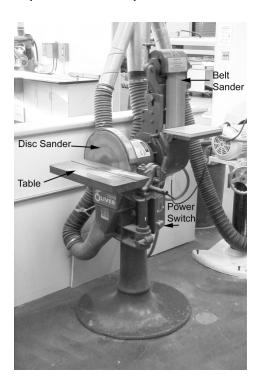
The disc sander consists of a reference table and a circular plate mounted to a motor shaft. A cloth or paper-backed abrasive disc is cemented to the plate. The diameter of the disc indicates the size of the machine, commonly 12". The combination sander includes a vertical belt sander as part of the machine.
