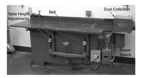
The edge sander is basically a large belt sander laid on its side. It is extremely useful for sanding long edges like face frames and frame-and-panel doors. Care must be taken to use it correctly, as abuse can ruin the belt, destroy your work, and injure you. Like the disc sander, it is a relatively safe machine, but can result in painfully skinned fingers if the operator is not careful.
