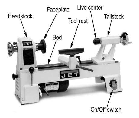
The lathe is used to make round or cylindrical shapes. Its primary components are the bed, headstock, tailstock, and tool rest. The work is rotated using a motor in the headstock; various tools are used at the tool rest to shape the work. The tailstock is used to support longer work at the opposite end of the bed. The lathe can be used to make a variety of turned objects, including table or chair legs, spindles, goblets, and bowls.
