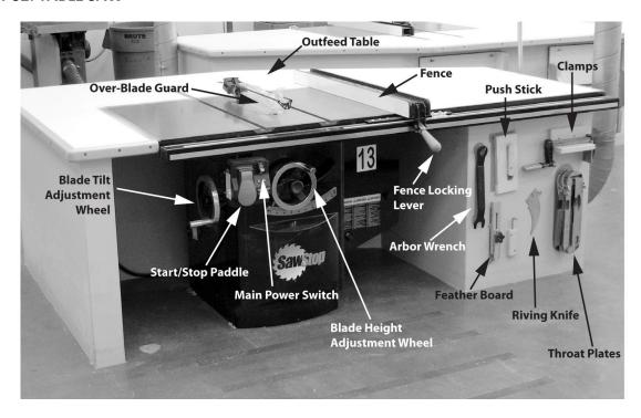
Although the table saw is one of the most useful machines in the wood lab, it is also one of the most dangerous. It can be used to accurately rip and crosscut lumber and sheet goods. The table saw can also be used for special operations including cutting dadoes and rabbets and for resawing. With the use of special jigs, joinery like tenons and box joints can be made. In addition, the blade can be tilted for cutting bevels and miters.
