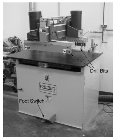
THIS IS A SPECIAL SETUP MACHINE; instructor approval is required for all operations.
