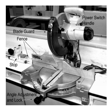
The miter or chop saw is the best tool in the lab for accurately crosscutting surfaced lumber to length. It is extremely useful for making all cuts from 90° to ±45°. The miter saw is one of the most dangerous machines in the lab. Use care in its operation.
