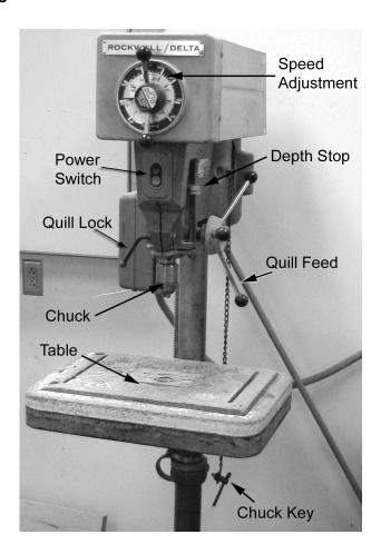
The drill press is an excellent machine for drilling accurate holes and is invaluable when drilling large holes. It consists of a motor/head assembly, chuck, and work table. Any uses other than drilling holes are **special setups** and must be approved by the instructor.
