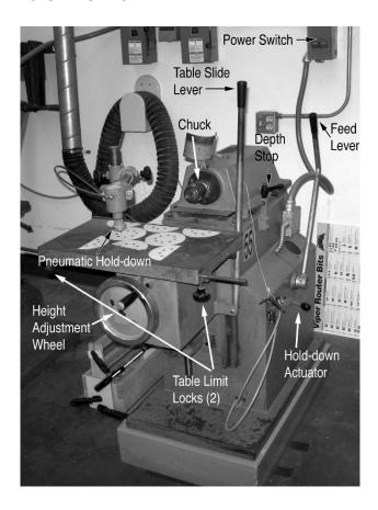
The slot mortiser is used for making slots or mortises. It is made up of a horizontally mounted motor/chuck assembly and an adjustable table. The table can be moved vertically and horizontally and the motor can be moved in and out relative to the base, making the mortiser very versatile for machining mortises.
