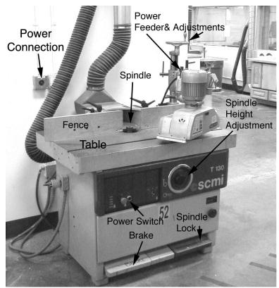
THIS IS A SPECIAL SETUP MACHINE; instructor approval is required for all operations.
