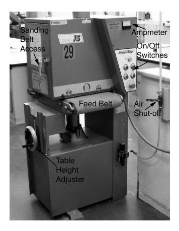
Wide belt sanders excel at smoothing lumber. A planer can be used for the same purpose, but planers can cause tearout on difficult grain. A wide belt sander will never cause tearout. Special precautions must be taken with the wide belt sander, however, as the machine is not as robust as a planer.
