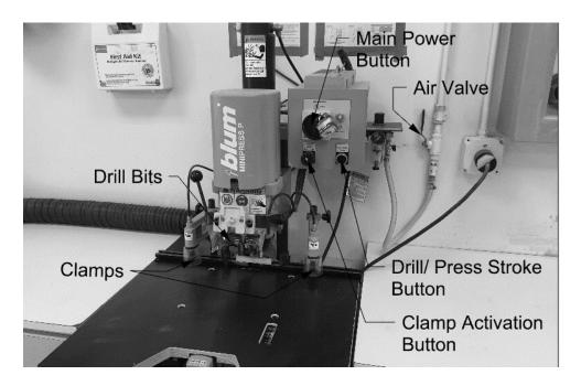
The hinge boring machine makes drilling holes for euro-style cup hinges a straightforward task. It drills the 35mm diameter cup and corresponding screw holes in one operation. Setup and operation are simple.
