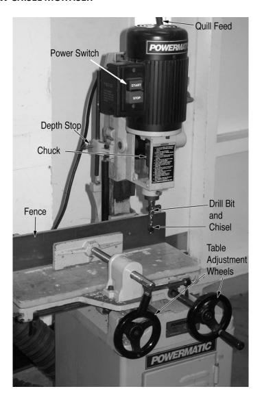
The hollow chisel mortiser is uniquely capable of making a square hole. It does so by forcing a hollow, four-sided chisel into the wood, and removing the encircled waste with a special drill bit. Due to the forces involved, a lot of heat is generated. Setup of this machine is critical; improper positioning of the chisel and bit can ruin the tool or the workpiece.
