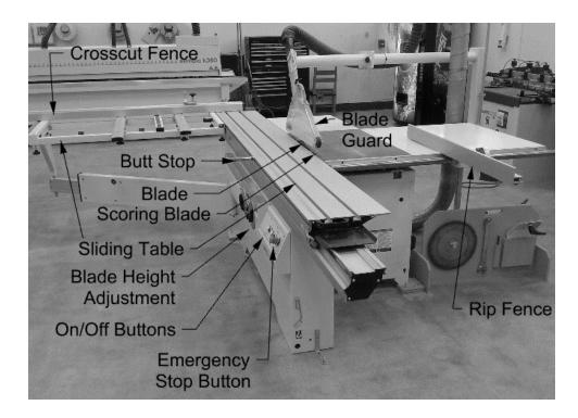
The sliding table saw is different from a typical table saw in that the portion of the table to the left of the blade slides back and forth. This sliding portion includes a crosscut fence and support structure for holding large panels, allowing sheet goods and other large pieces to be ripped or crosscut easily. The saw incorporates a scoring blade in front of the main blade to eliminate tearout or chipping on the underside of the cut.
